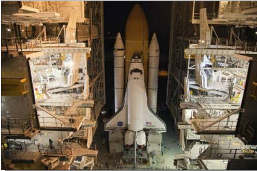
The space shuttle Discovery was rolled back to the Vehicle Assembly Building at NASA's Kennedy Space Center in Florida to allow crews to take X-ray scans beneath the foam insulation of all 108 support beams on Discovery's external tank. Photo: NASA/Frank Michaux
