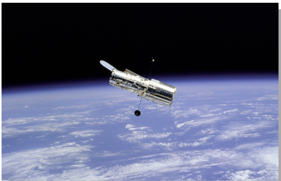
With a mass of 11 tons and 43 feet (13.2 m) long, the Hubble Space Telescope has been peering into the depths of the universe since 1990. Here it's seen in February 1997, during the second of five Space Shuttle servicing missions. NASA
