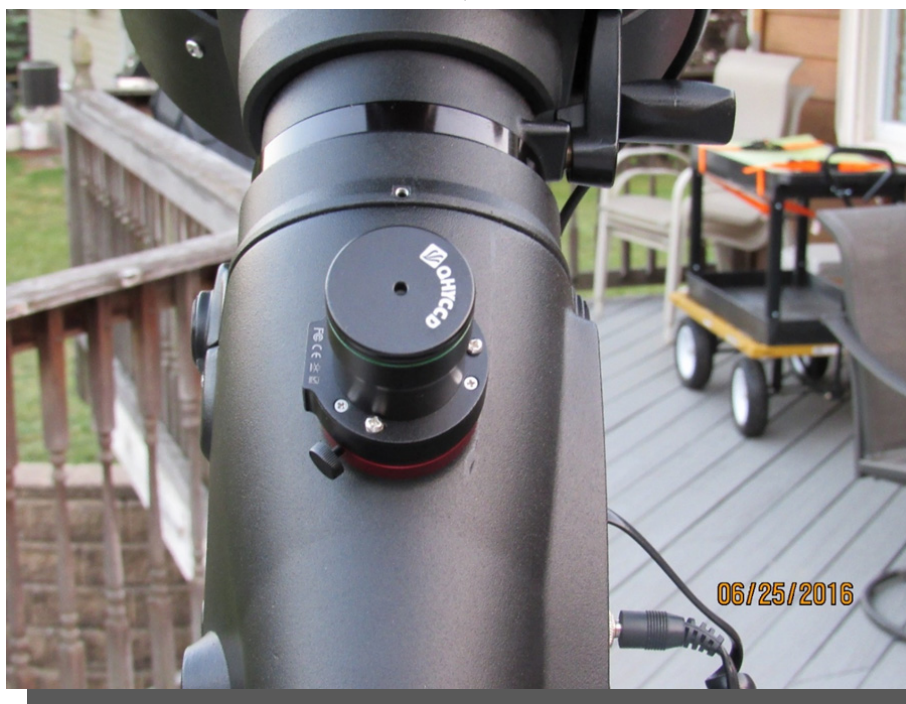
Figure 2. PoleMaster Installed on CGEM-DX
