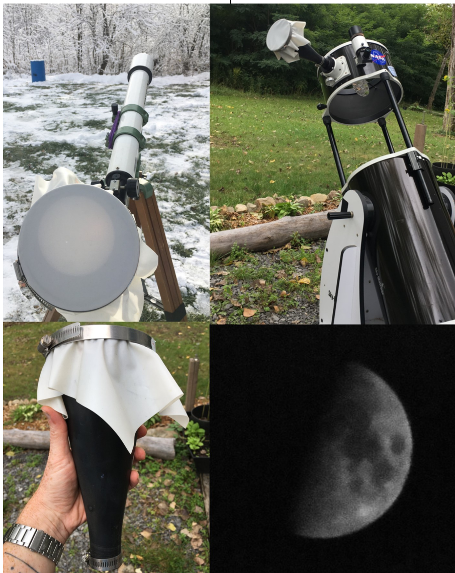
Sun Funnels in action! Starting clockwise from the bottom left, a standalone Sun Funnel; attached to a small refractor to observe the transit of Mercury in 2019; attached to a large telescope in preparation for evening lunar observing; projection of the Moon onto a funnel from a medium-size scope (5 inches).
